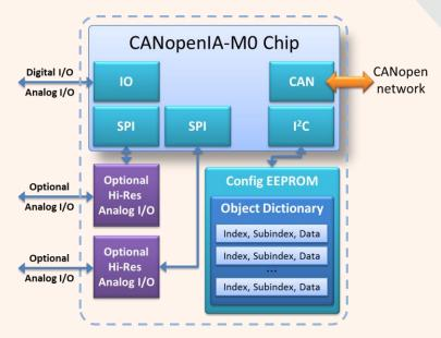
Configurations can be generated and loaded using the provided CANopenIA-M0 setup utility. The chip's configuration gets stored in an EEPROM. Configurable parameters include:
